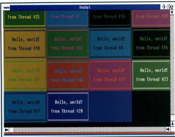
Hello, world is running in a Presentation Manager window. Each frame has a different foreground and background color because an attribute byte for each frame has been added to the FRAME data type.
